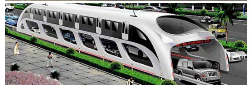
This is a design for a bus in China that could drive over other cars
