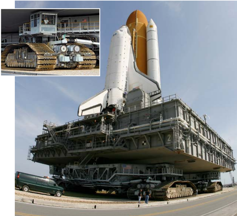
This vehicle moves space shuttles at a top speed of .9 miles per hour (1.4 kph).
